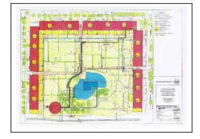
This project was recognised as an exemplary model of an ecological project in the Habitat II Conference in Istanbul in 1996. The storm water runoff from the roofs is stored in a 600 m<sup>3</sup> cistern and reused for irrigation and for the regulation of a rain water pond.
